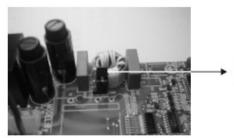
JUMPER is used as a voltage selector
